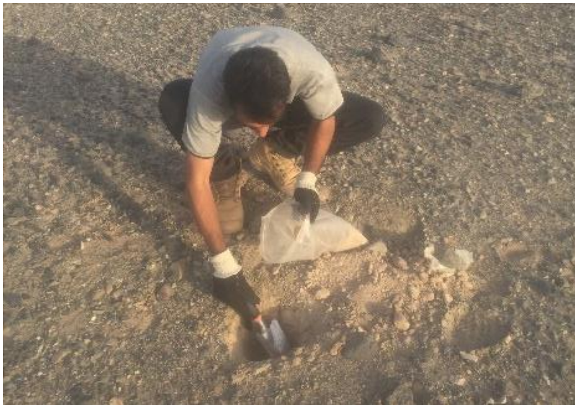
Soil sampling using SS Bailer at S2-22
