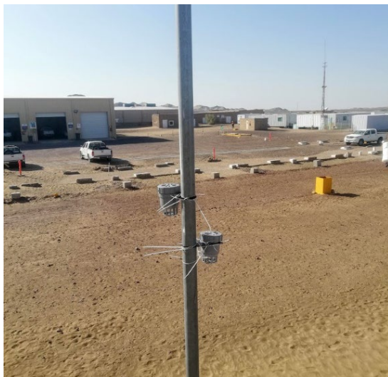
Diffusion tubes installed at A1-23
