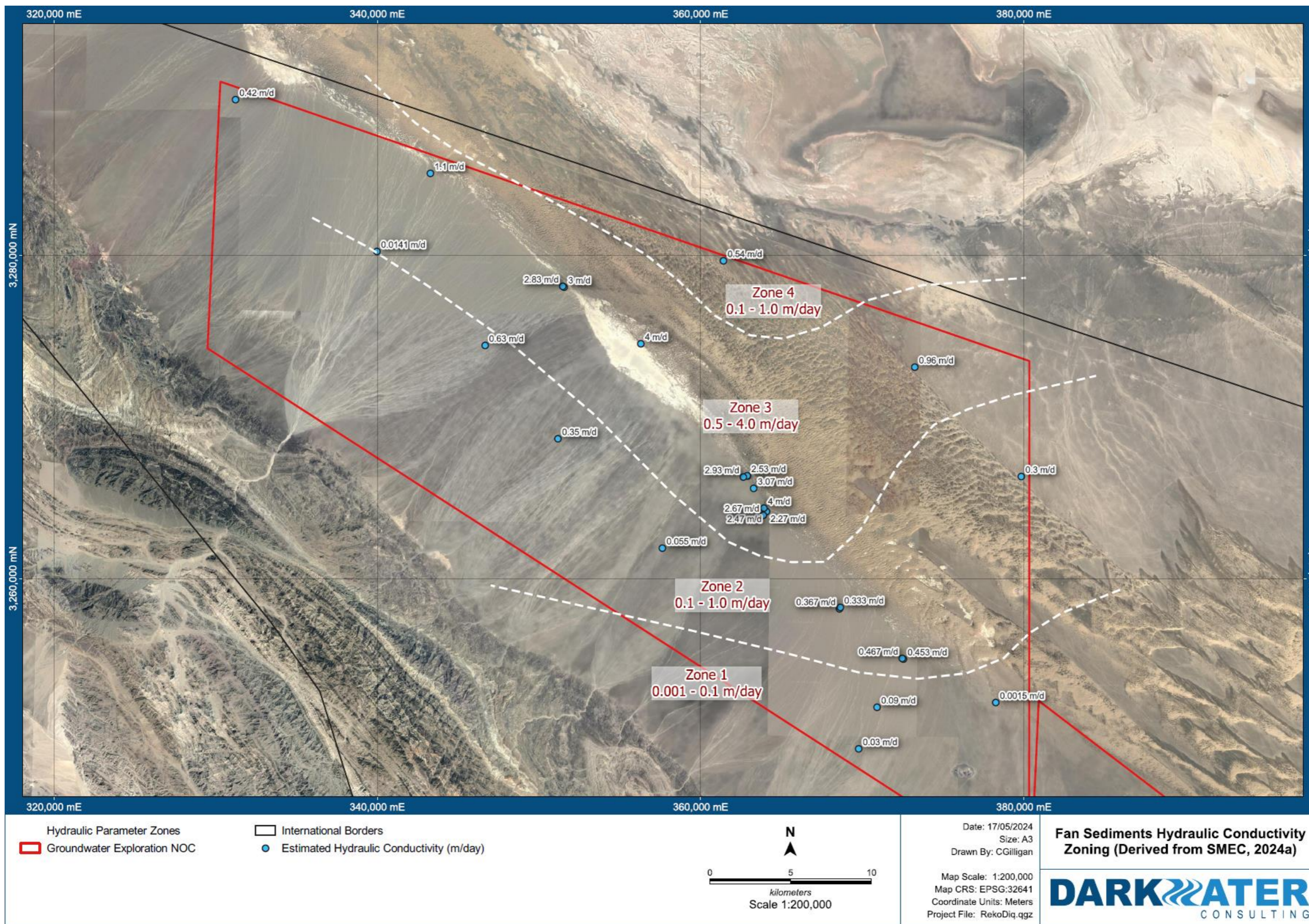
Figure 15: Hydraulic Conductivity Zoning (Derived from SMEC, 2024a)
