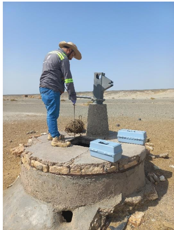
Team collecting water sample from Dug well at W12 – Mashki Chah
