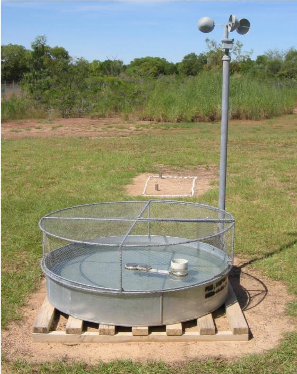
Class A Evaporation Pan with bird guard (Source: Wikipedia)
