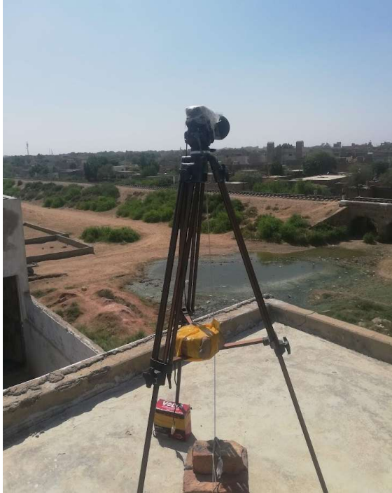
Noise meter installed at N21
