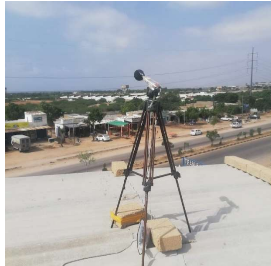
Noise meter installed at N24
