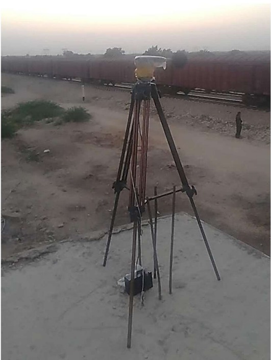
Noise meter installed at N22
