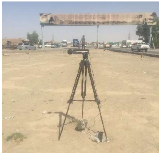
Noise meter installed at N4
