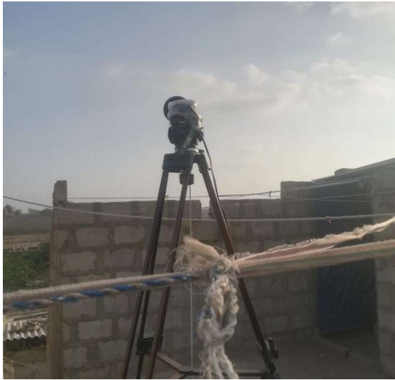
Noise meter installed at N23
