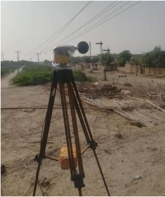
Noise meter installed at N16
