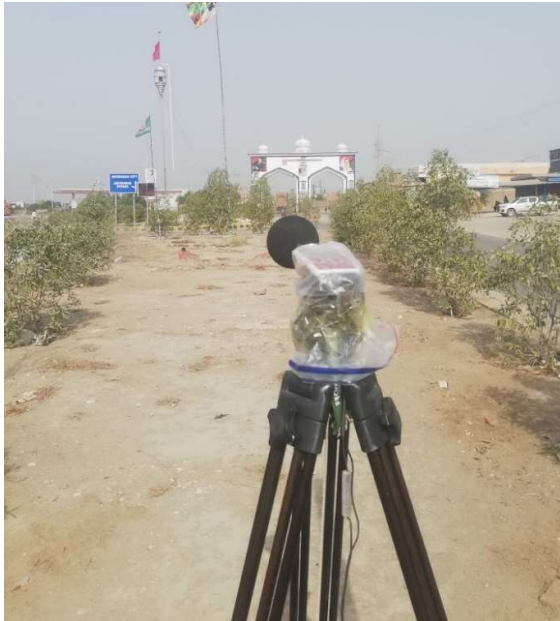
Noise meter installed at N17
