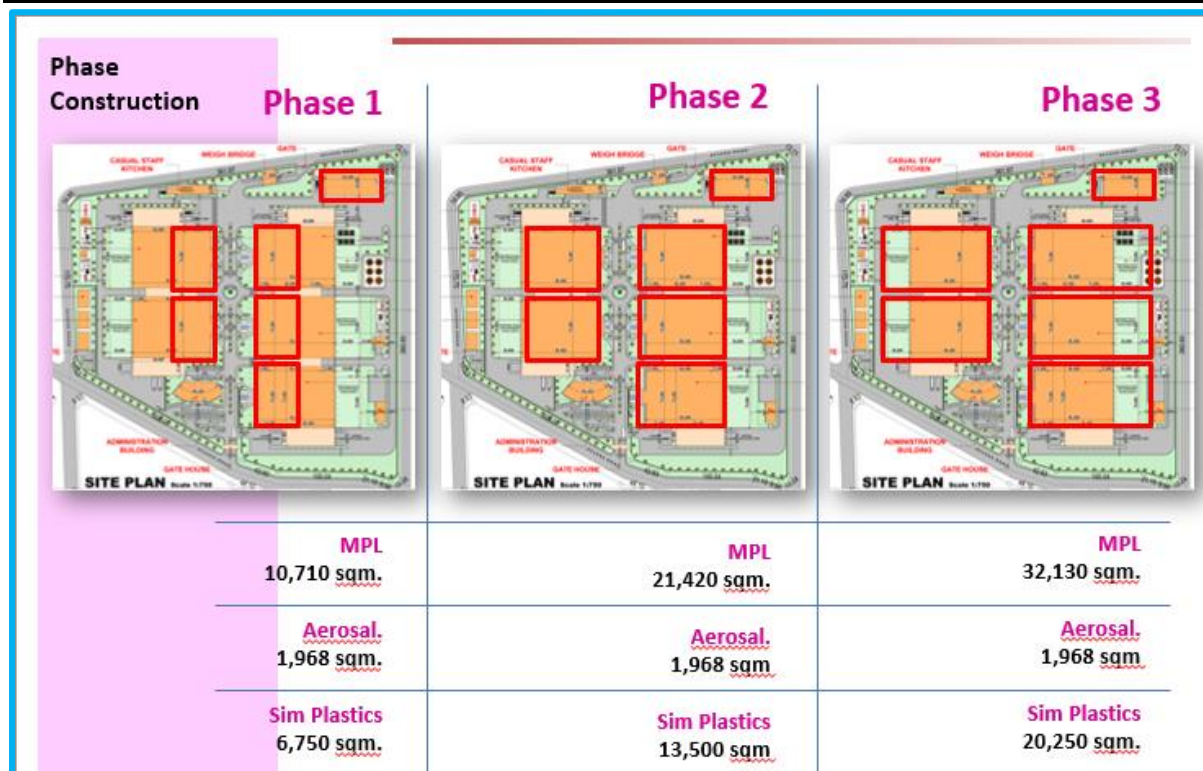
Figure 2.4-6: Project Phasing During the Construction
