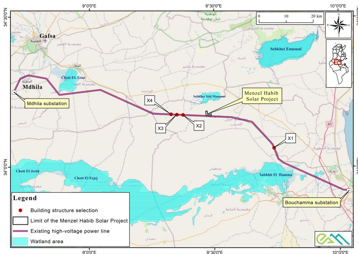
Figure 7.54 - Location of structures identified along the existing 150 kV transmission Bouchamma - Mdhilla (less than 14 m on either side of the line)
