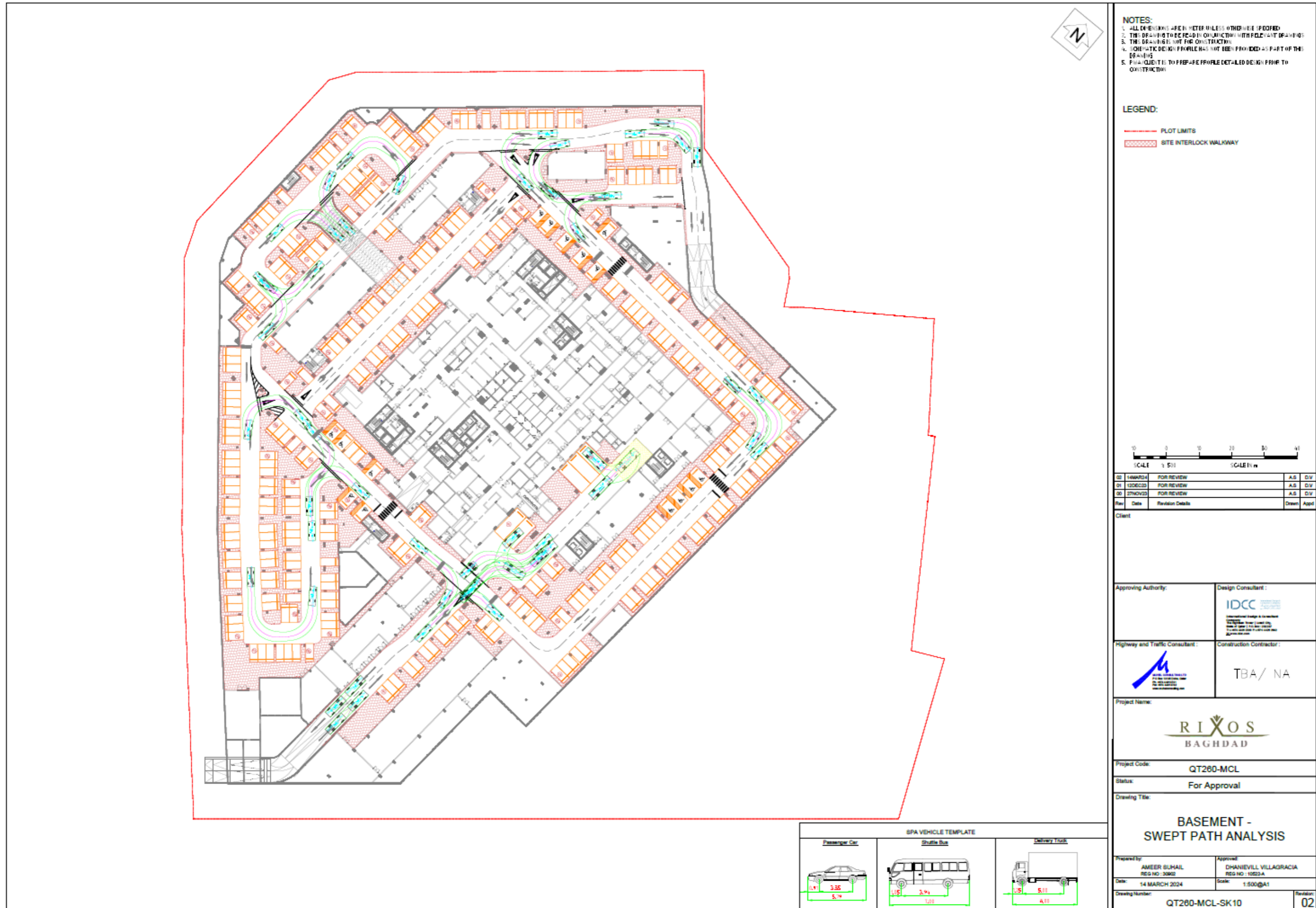
Figure 2-7: Basement Parking Swept Plan
