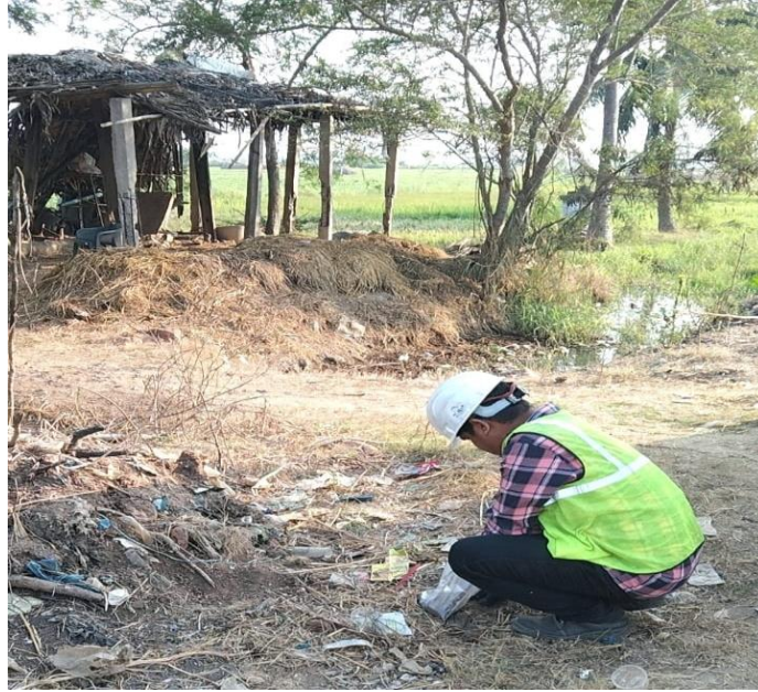
Figure 3-16 Soil sample collection
