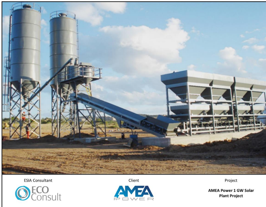
Figure 8: Typical Mobile Batching Plant
