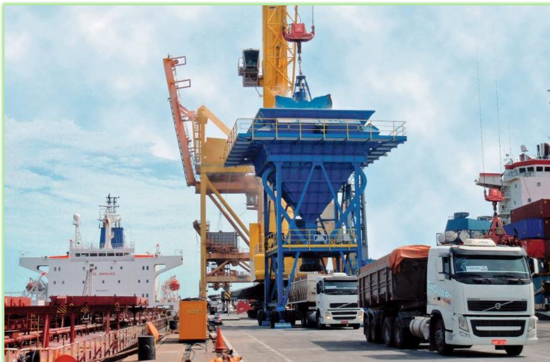
Figure 3-17: Typical Eco Hopper used for discharging bulk materials at the Port
