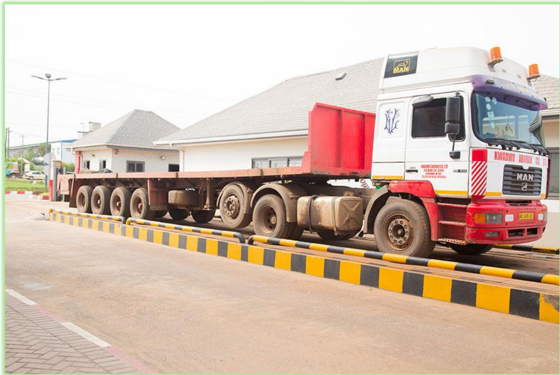
Figure 3-13: An unloaded truck being weighed on the weighing bridge
