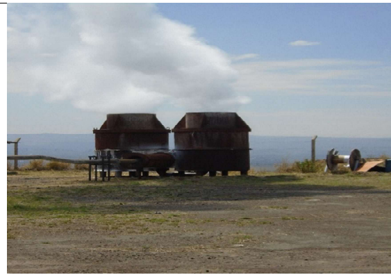
An existing discharge well at Menengai well 3 site. These are some of the activities contributing to the existing noise and H 2 S levels within the caldera
