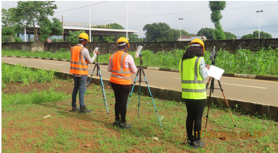
Figure 4-1: Air Quality and Noise Monitoring in the Police Training Ground
