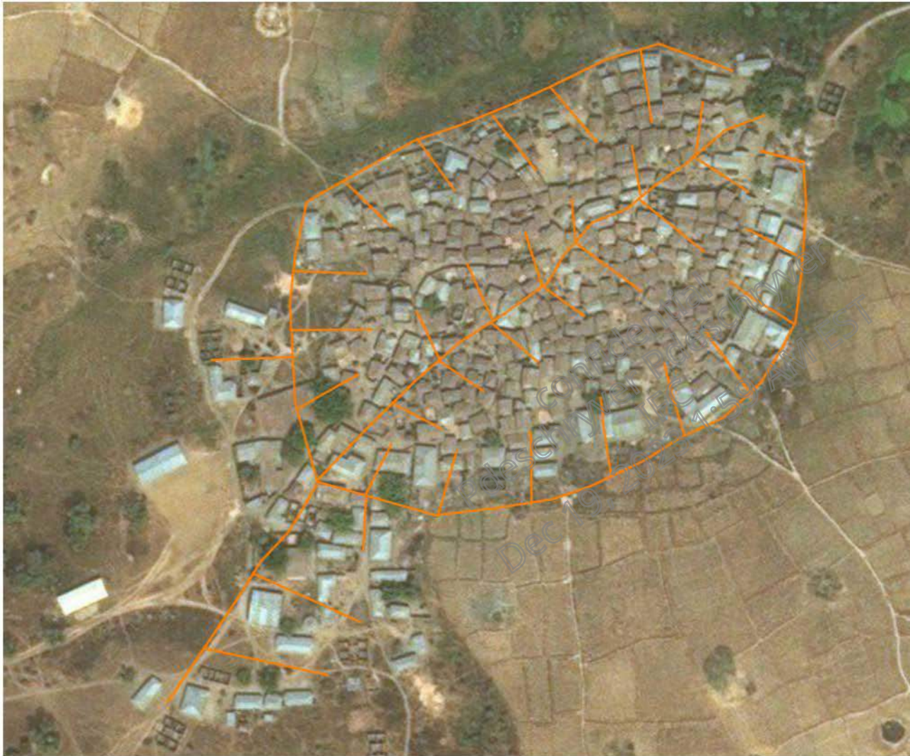
Figure 3.16: Typical layout for power distribution within the households in the beneficiary communities
