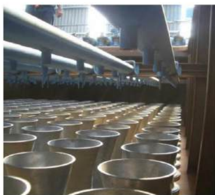
BAG FILTER – Internal view
