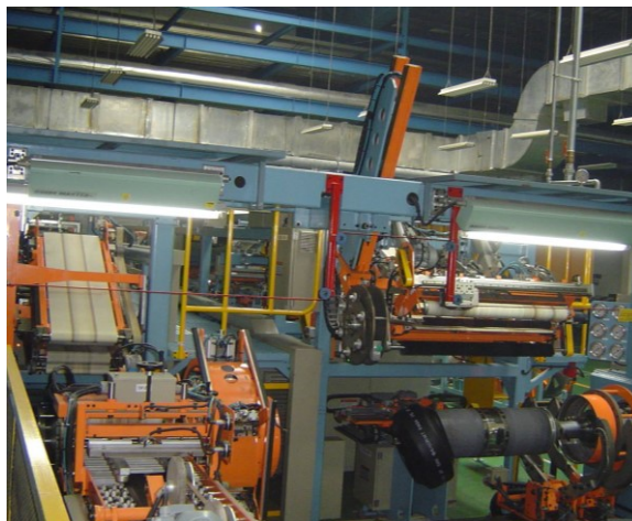
Figure 2.13: A view of One-Stage Buiding Machine
