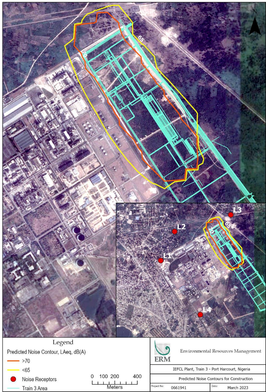
Figure 8-9 Predicted Noise Contours during the Construction Phase
