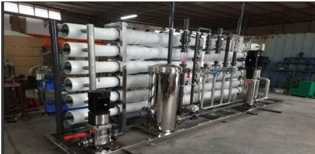
Complete containerized RO plant
