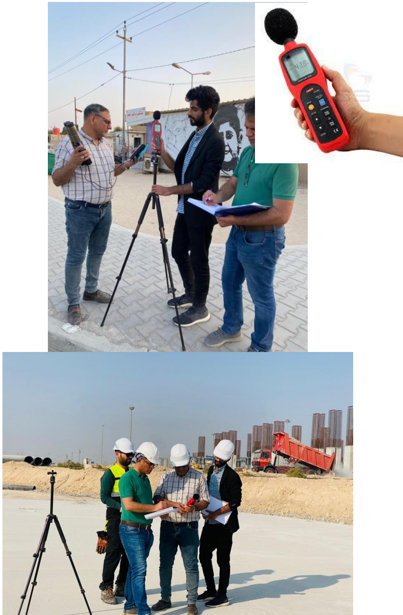
Figure 8-2: Noise meter used for monitoring at 6 locations (4 locations at facility fence and 2 locations at offsite sensitive receptors) (Picture to the right is monitoring at project site and at the left is monitoring at sensitive receptor (Hospital))
