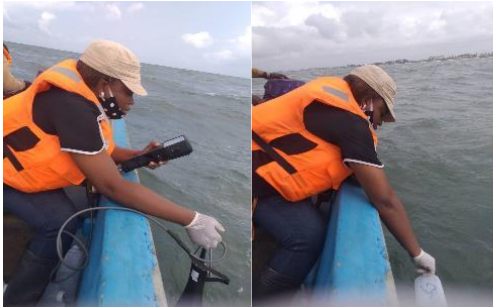
Plate 3: Surface water in-situ sampling and sample collection
