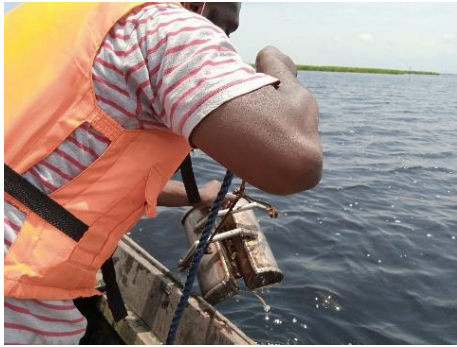
Plate 5: Grab sampling from the bottom of the Lekki Lagoon
