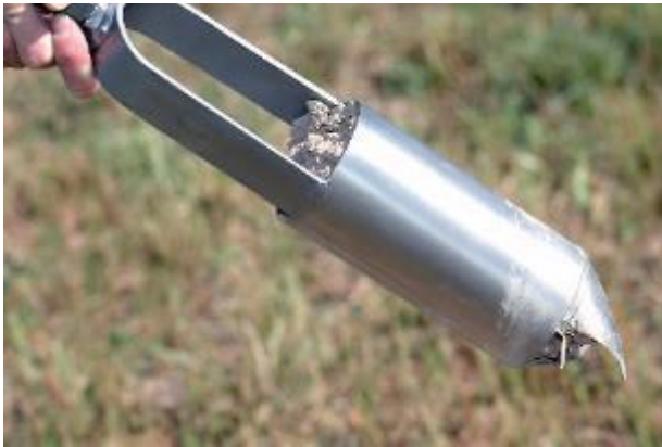
A: Soil Auger for soil burrowing
