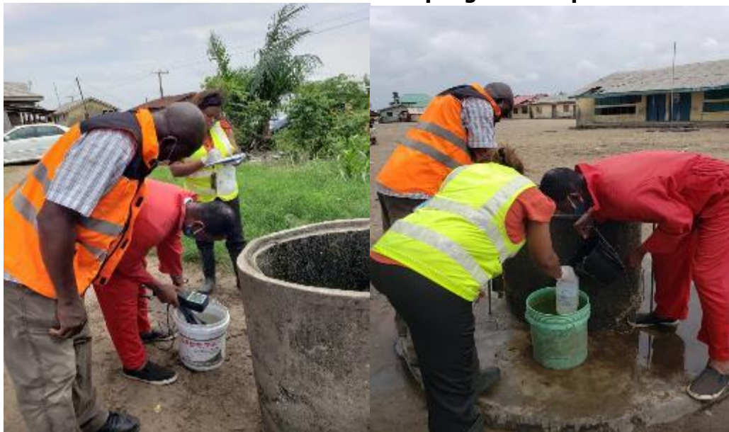
Plate 4: Groundwater in-situ sampling and sample collection
