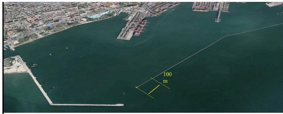
Figure 3 Shortening the main breakwater for 100 m
