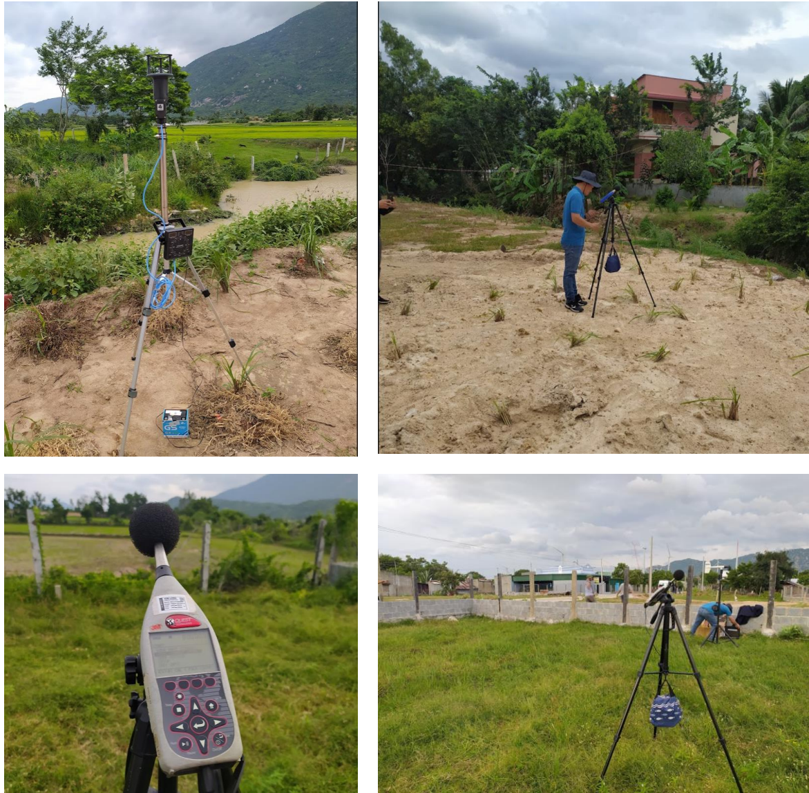
Figure 7.17 Site Setup for Noise Monitoring Location N1 (above) and N2 (below)
