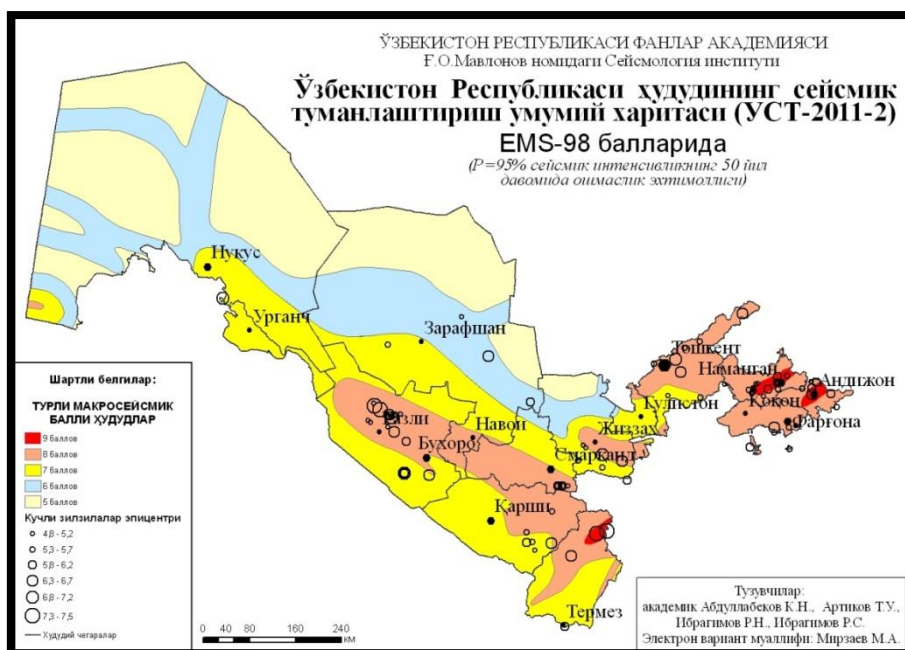
Figure 14 Seismic regionalization of the Republic Uzbekistan (yellow 5 ball, dark yellow 7, and blue 6ball)
