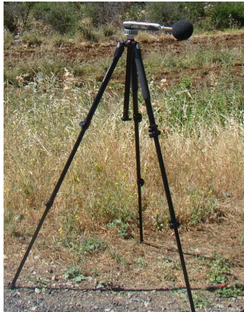
Noise Meter Siting at Appropriate Height
