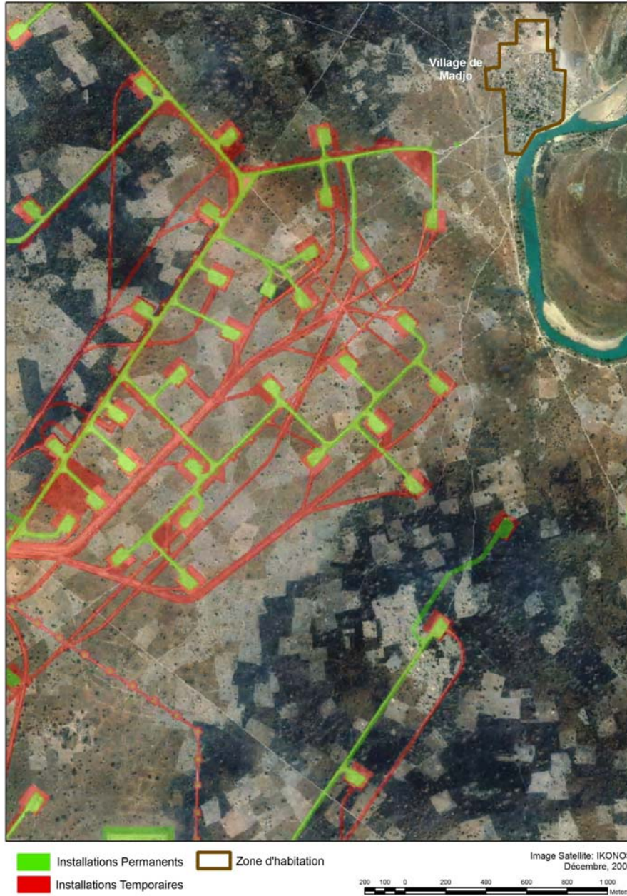
Madjo Installations (well pads and flowlines)
