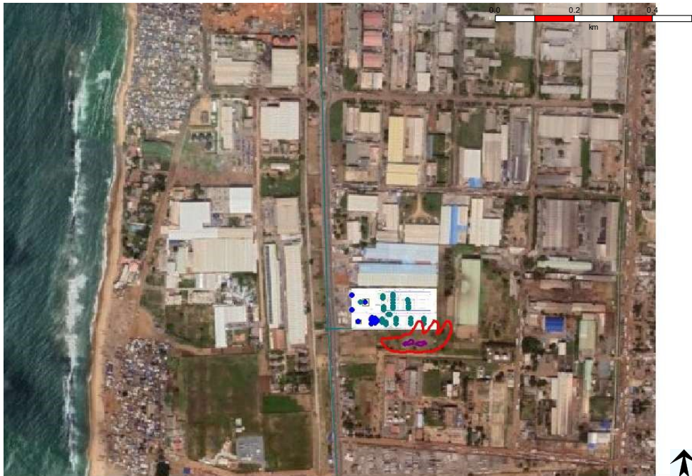
Figure 4-8: Exceedance frequency maps for Pool fire at 37.5 kW/m 2
