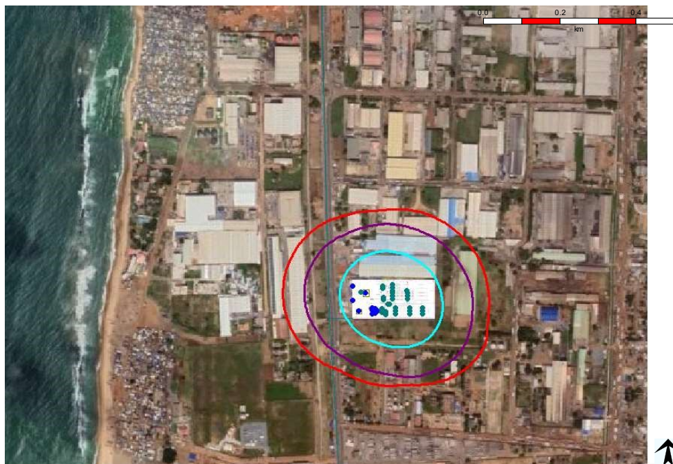
Figure 4-7: Exceedance frequency maps for Jet fire at 37.5 \text{ kW/m}^2
