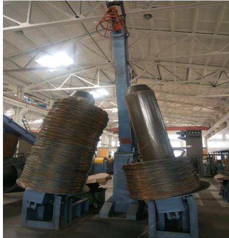
Plate 1: Vertical Dual Station Pay-off with scale collecting boxes
