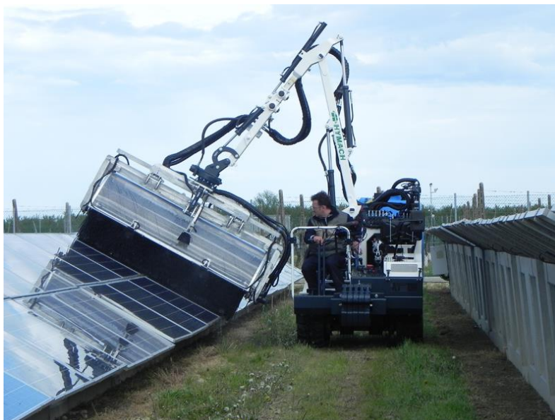
Figure 69. Wet cleaning system
