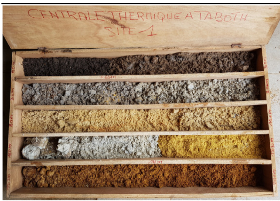
Figure 6.4 Coupe de sol, carottage SC1
