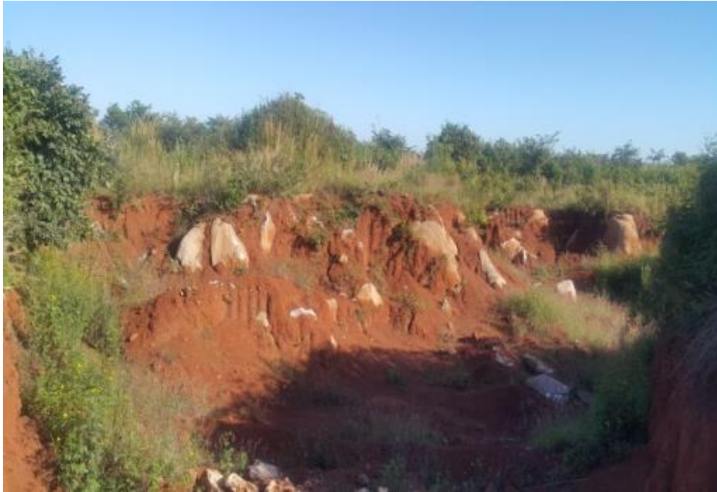
Photo 4.4: Exposures in a burrow pit on the northern side of the project area showing varying soil depth and rock boulders floating in soil mass. The pit is located about 500 metres to the north of the project site.
