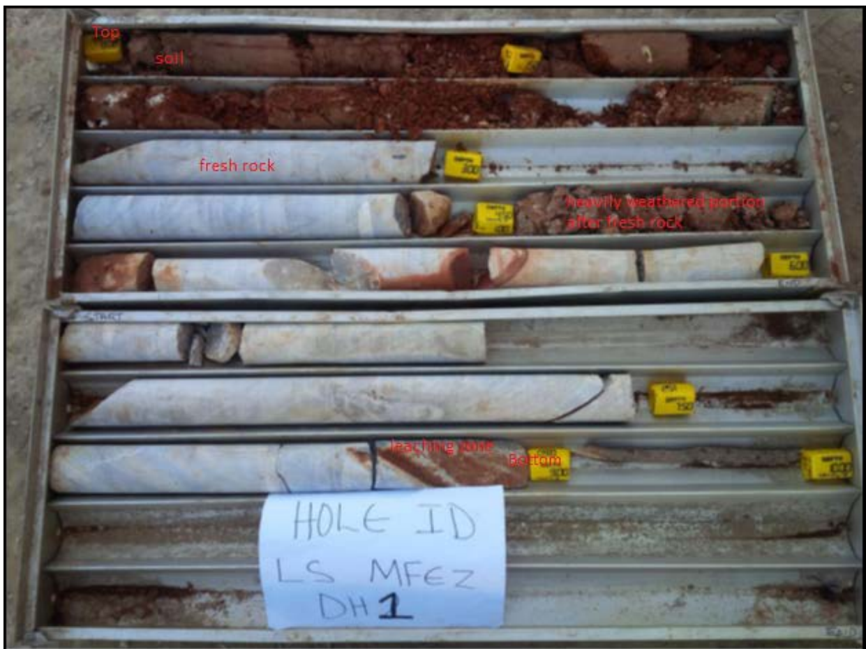
Photo 4.2: Uncertainties in drilling profiles, heavy weathering after fresh rock (AMC, 2015e)
