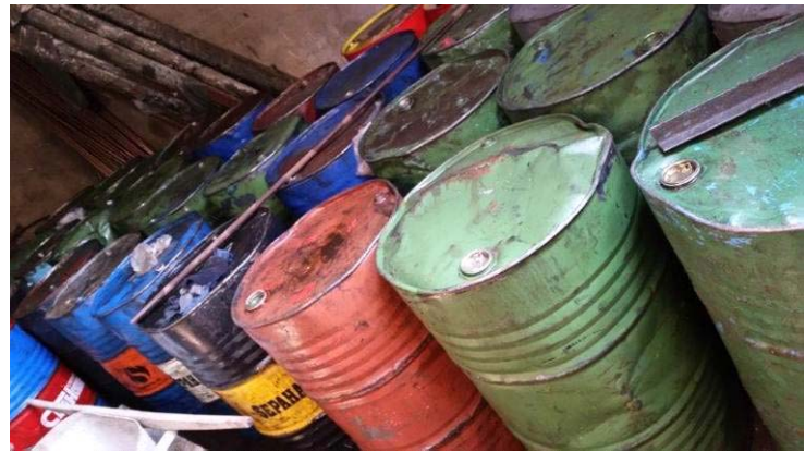
Photo 75: Oil, gasoline and other substances stored without labelling in rooms without any ventilation
