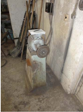
Photo 51: Dangerous tools without workers' protection
