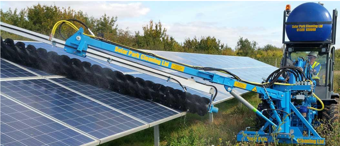
Figure 71: Wet cleaning system
