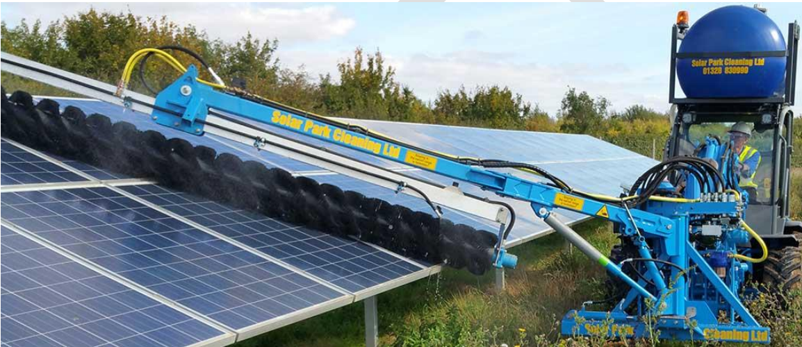
Figure 64. Wet cleaning system
