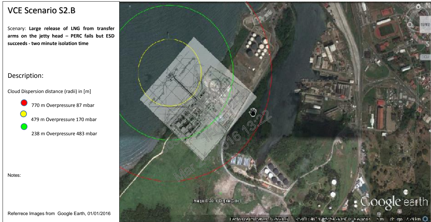
Figure 4-2 Overpressure Results (VCE) for Scenario S-2.B
