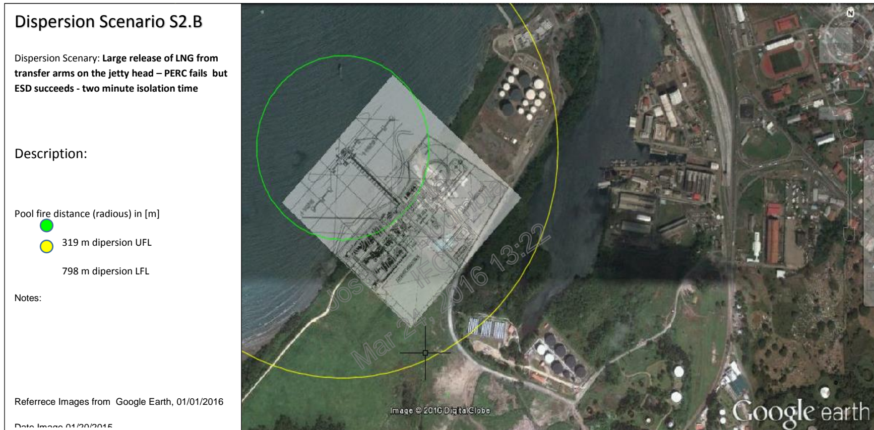
Figure 4-3 Flammable Gas Dispersion for Scenario S-2.B
