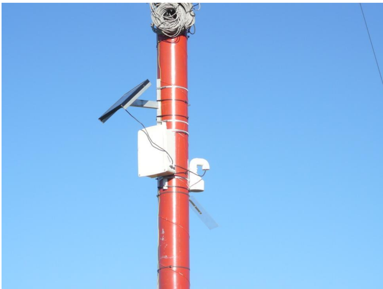
Figure 4: White weather box (with Anabat detector inside) and solar panel mounted on tubular mast.
