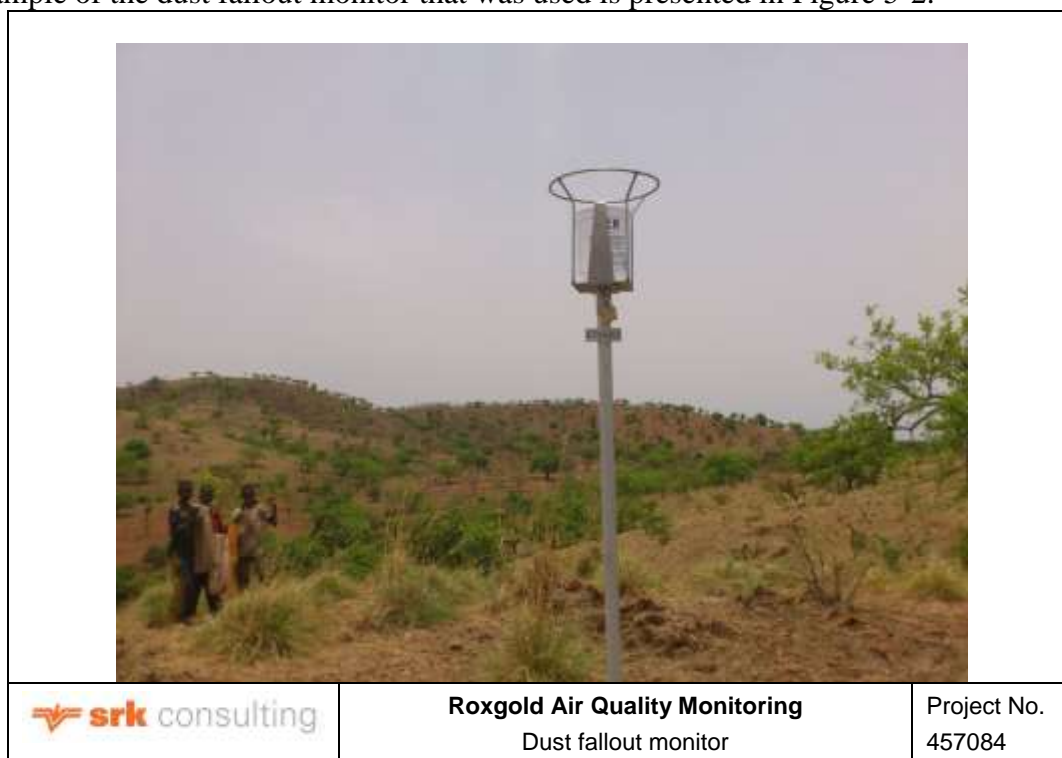
Figure 5-2: Dust fallout monitor installed within the Roxgold mine concession.
