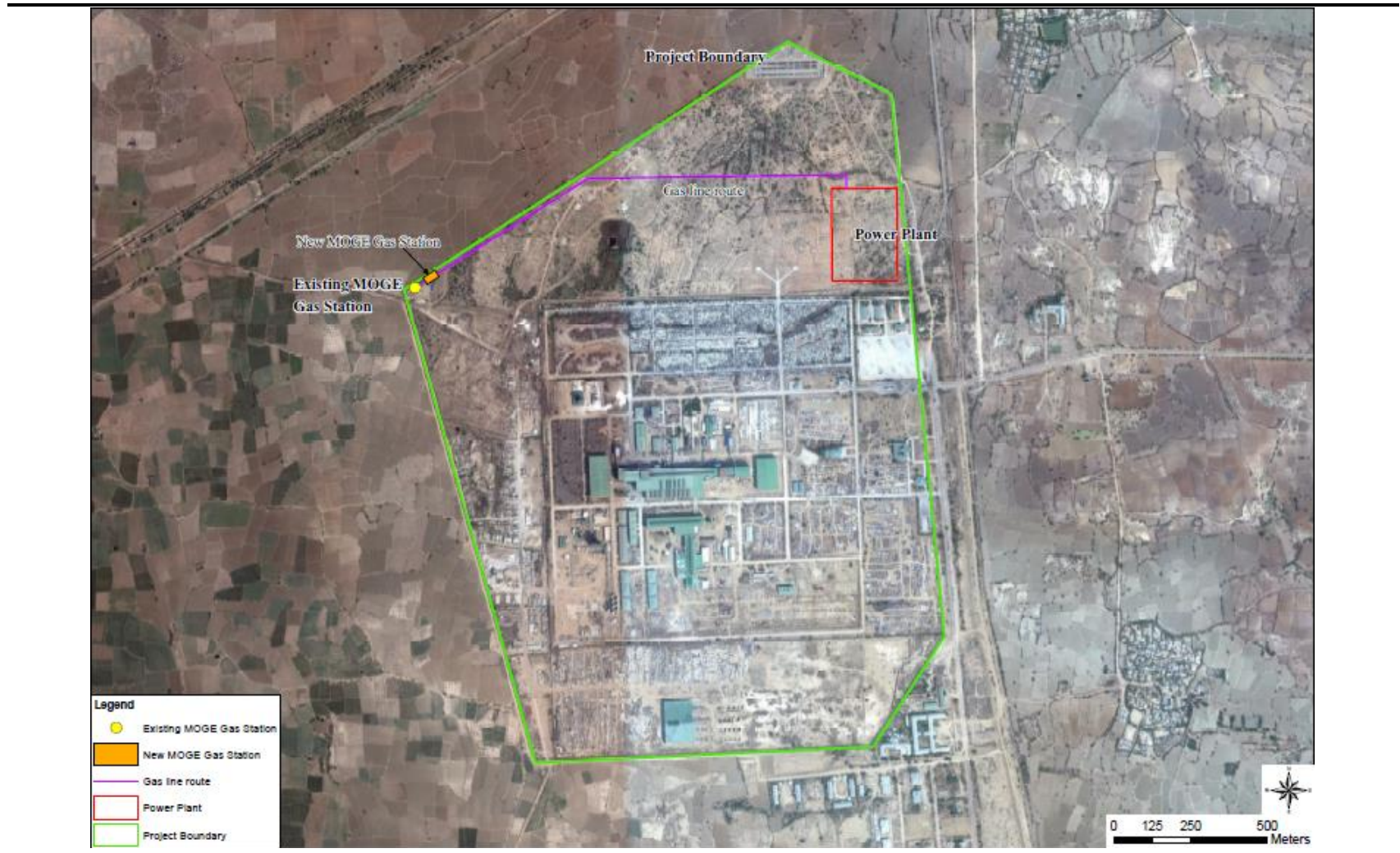
Figure 2.1 Proposed Pipeline Alignment (Fuel Gas Source)
