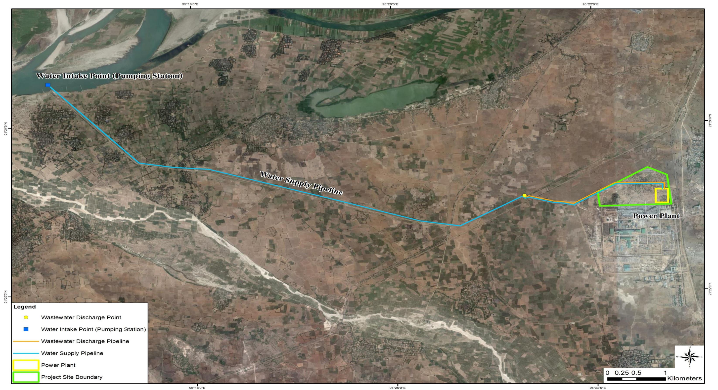
Figure 2.9 Proposed Alignment of Water Supply Pipeline from the Power Plant to the Ayeyarwady River Water Intake Point and Wastewater Discharge Pipeline
