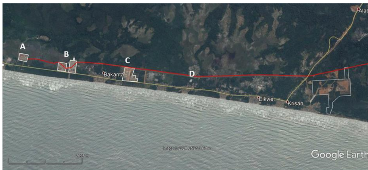
Figure 7-8 Overview map identifying other major oil and gas developments and activities in the study area and extending to the west. Recent industrial facilities include A. The Ghana gas accommodation camp; B. The Ghana gas batching plant (left) and processing facility (right); C. Quantum gas facility, and; D. The Ghana Gas Export pipeline (red). Other industrial projects nearby also include the Nzema Gold Mine located in Nkroful (approximately 4km North of Esiama) (image source: Google Earth)
