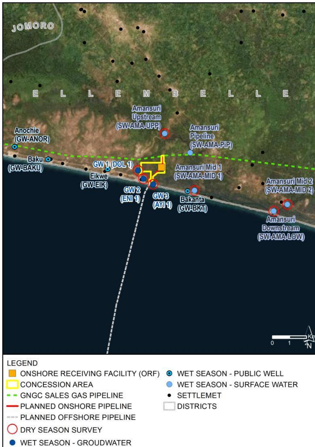
Figure 6.4 Surface and groundwater sampling points
