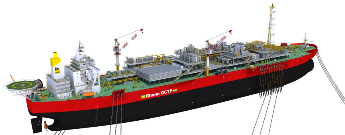
Figure 2-14 Pictorial of double balcony FPSO
