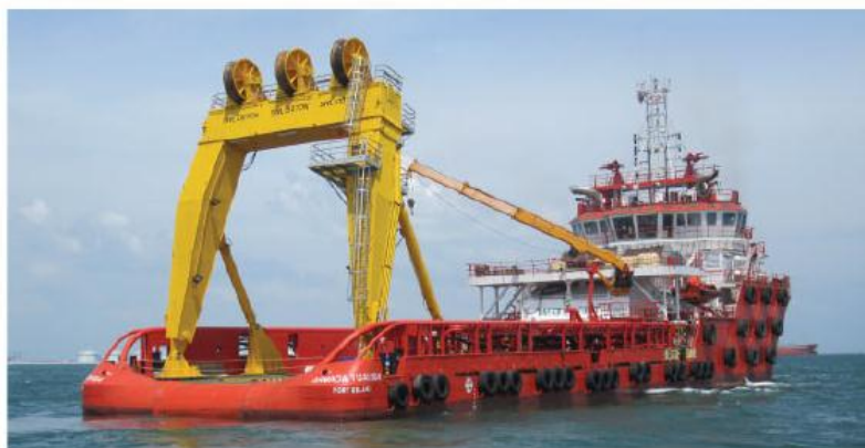
Figure 2-18 Example of a Vessel Anchor Handling
