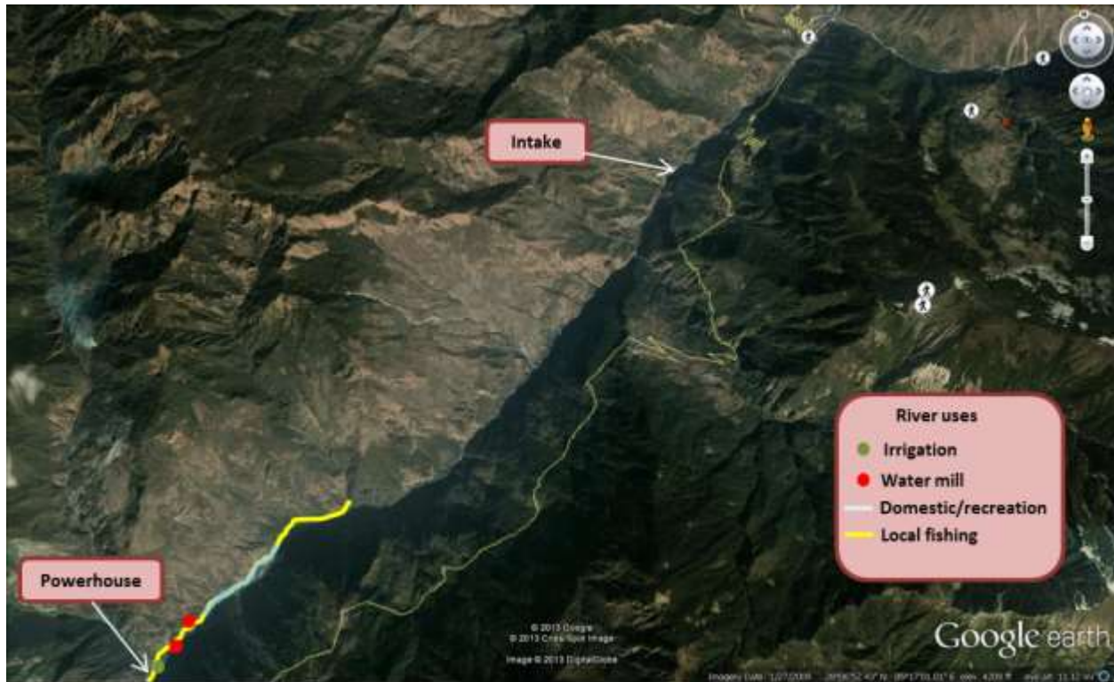
Figure 5-5: River uses in the diversion reach of the Project
