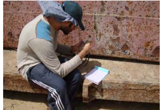
Photograph 06: Field testing for pH, TDS, salinity, and temperature during sample collection
