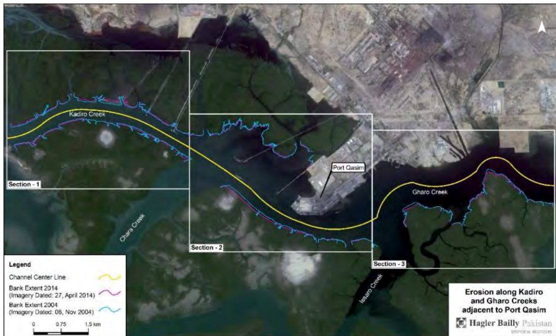
Exhibit 4.41: Erosion along the Current Navigation Channel and Anticipated Extension
