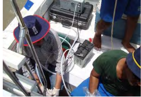
Photograph 02: Seawater quality sampling in progress with the bladder pump
