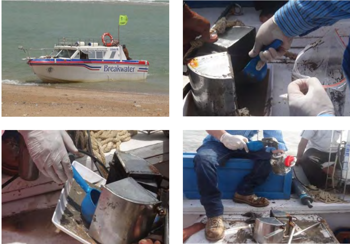
Benthic Sediment Sampling techniques used for collection of bottom sediments to evaluate MBI.
