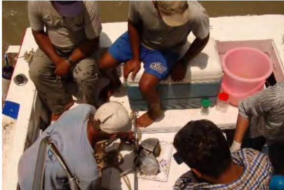
Photograph 01: Sample extraction from the Ponar grab sampler
