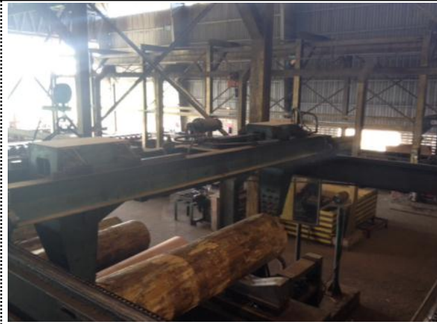
Photo 2: Automated log splitting operation. Limited manual interventions in operations
