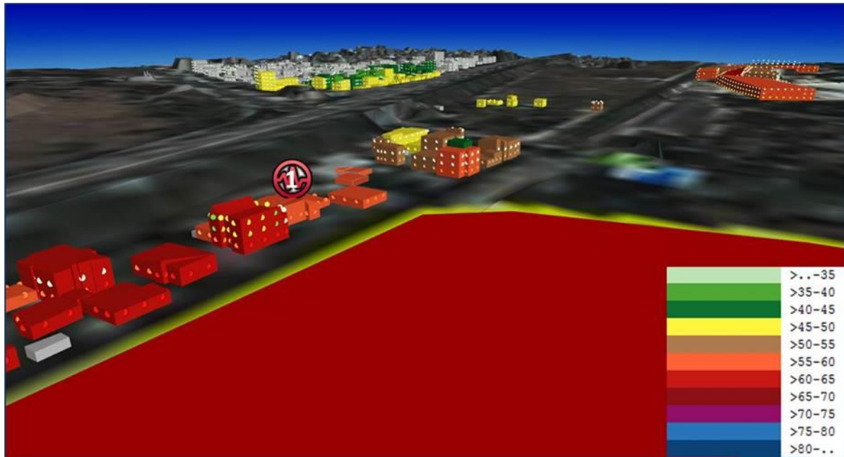
Figure 10-10: Facade noise level calculations, measurement location 1, Phase 1
