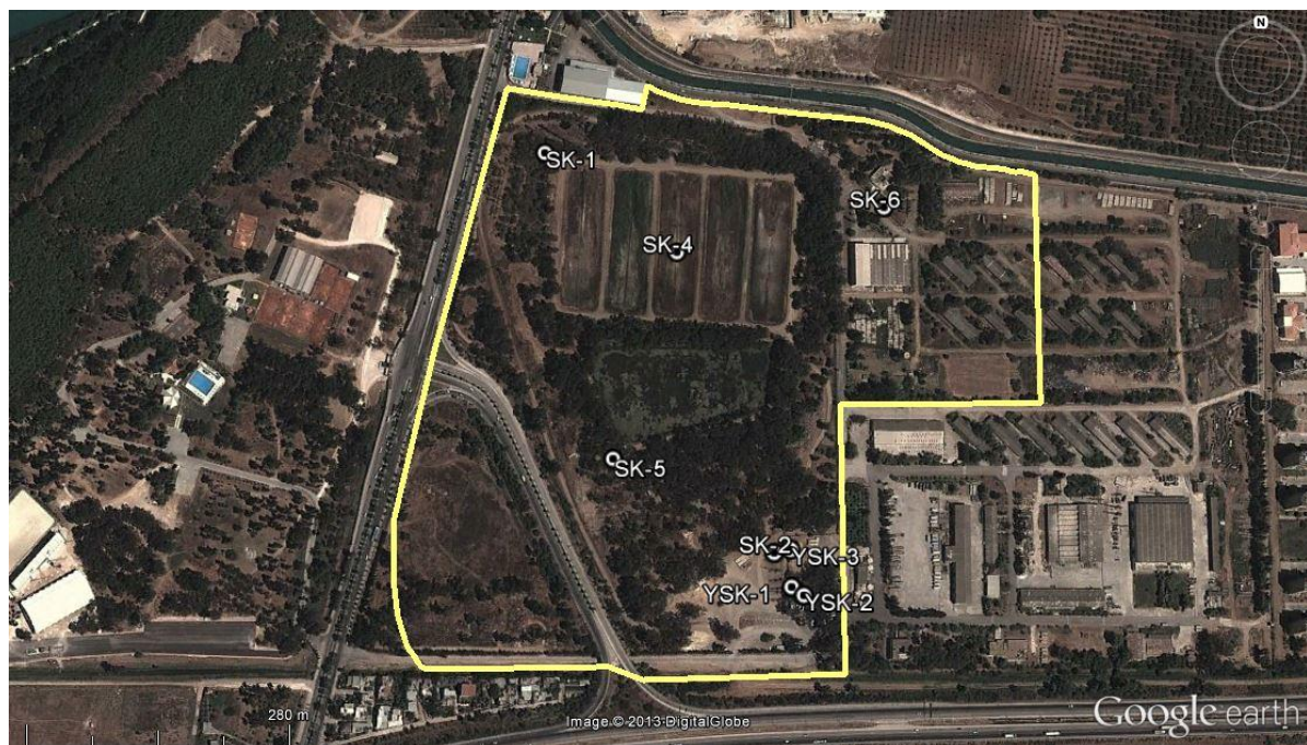
Figure 6-11: Sampling locations (SK-1 and SK-2 (20 m groundwater monitoring wells), SK-4 through SK-6 shallow boreholes (maximum depth 1.5 m), YSK-1 through YSK-3 shallow soil samples in the DSI maintenance area)
