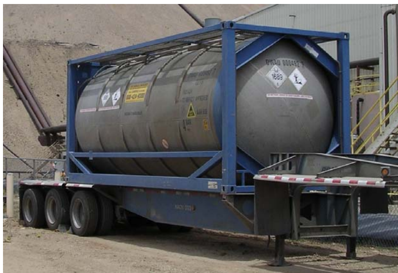
Figure 9.3-14: Typical Stainless Steel ISO Delivery/Mixing Container (Source: ENVIRON)
