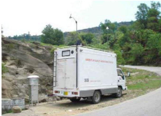
Fig 3: Ambient Air Quality Monitoring at Power House Site
