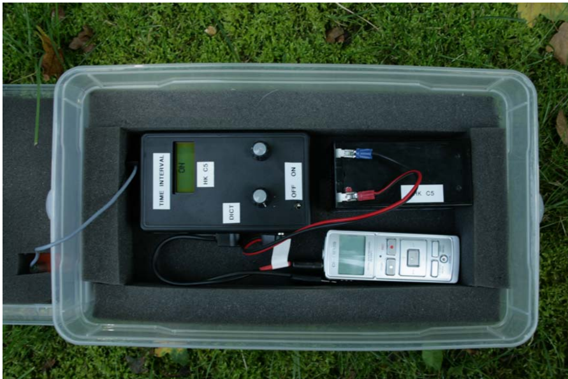
Figure 3.1: Bat-box. Left: detector with cable to microphone. Right: energy supply and digital audio recorder.
