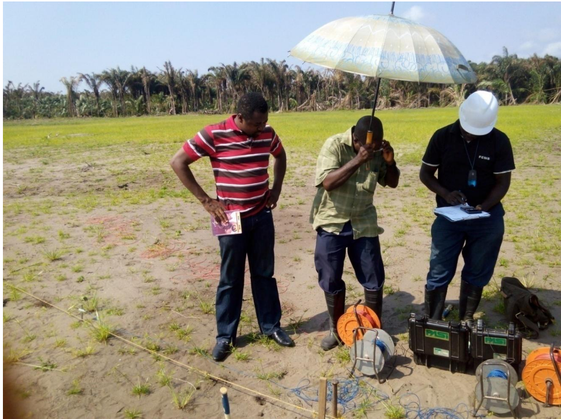
Plate 4-4: Geophysicists taking VES at one of the sampling stations with FMEEnv Official witnessing
